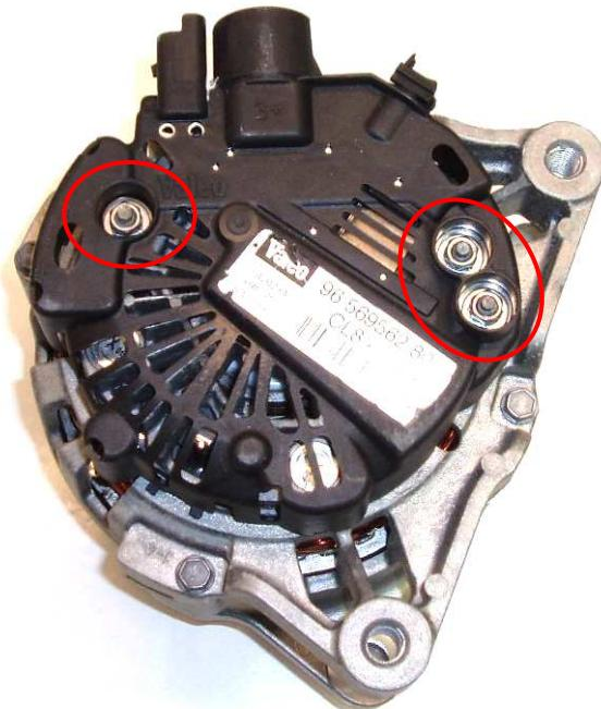
2 - Apply some seal paste (« caf ») on 3 poles shown on the picture below and the body as well, to reduce vibrations :
