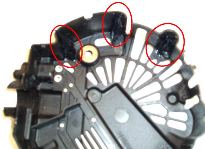
4 - Cover the alternator with his bonnet and torque the three nuts :
